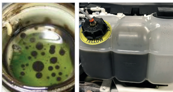
Impurities in the cooling circulation system
